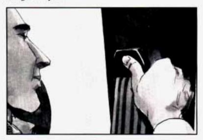
To move it down, push in at the top of the arrows and move the height adjuster to the desired position. You can move the adjuster up just by pushing up on the shoulder belt guide. After you move the adjuster to where you want it, try to move it down without pushing in to make sure it has locked into position.
